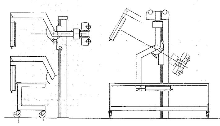
The design of the trolley must permit the use of the cassette holder in horizontal position under the trolley in such a way that the distance between the table top and the film plane does not exceed 8 cm. In this position it must be possible to use the trolley as a floating-top table, so that the longitudinal midline of the trolley can be offset no less than  $\pm$ /- 12 cm from the midline of the cassette holder.
