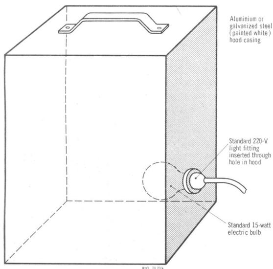
*Desiccators.* The principle employed in the standard glass, plastic or metal desiccator is different from that of the heat cabinet in that the drying of the air is brought about by the physical or chemical removal of the water from the air by drying agents; there is no rise in temperature. In this way condensation is prevented and thus corrosion and propagation of fungus are inhibited.
