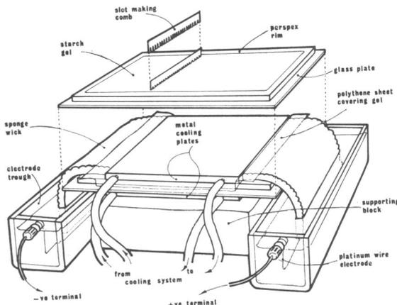
Fig. 1. Apparatus for starch gel electrophoresis.
