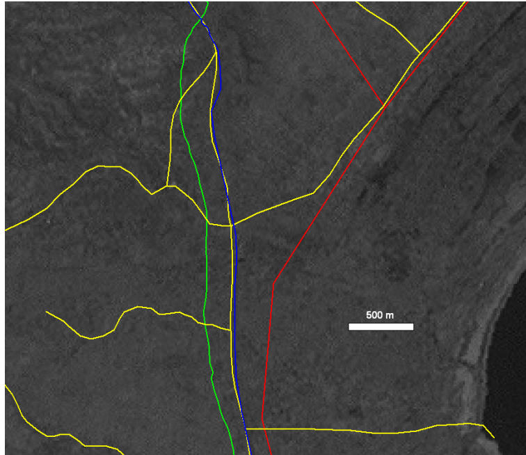
Figure 3 - Extract of the road network for Malawi with in Yellow: the one coming from the Survey Department; in Green: the one coming from the National Statistical Office and in Red: Global insight database; Blue: the one extracted from the satellite image.
