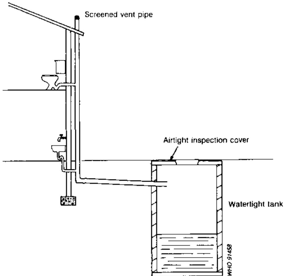
**Fig. 6.40. Manually flushed chemical toilet**
