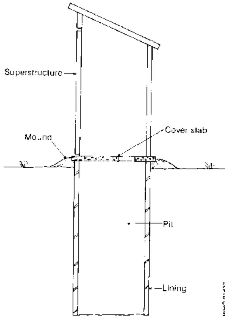
The cover slab should be raised at least 150 mm above the surrounding ground to divert surface water away from the pit. Commonly, the cover slab sits directly on the lining, but if the lining is made of very thin material, such as an old oil drum, a concrete foundation beam may be necessary to distribute the load of the slab to the lining and surrounding ground (Fig. 6.4).
