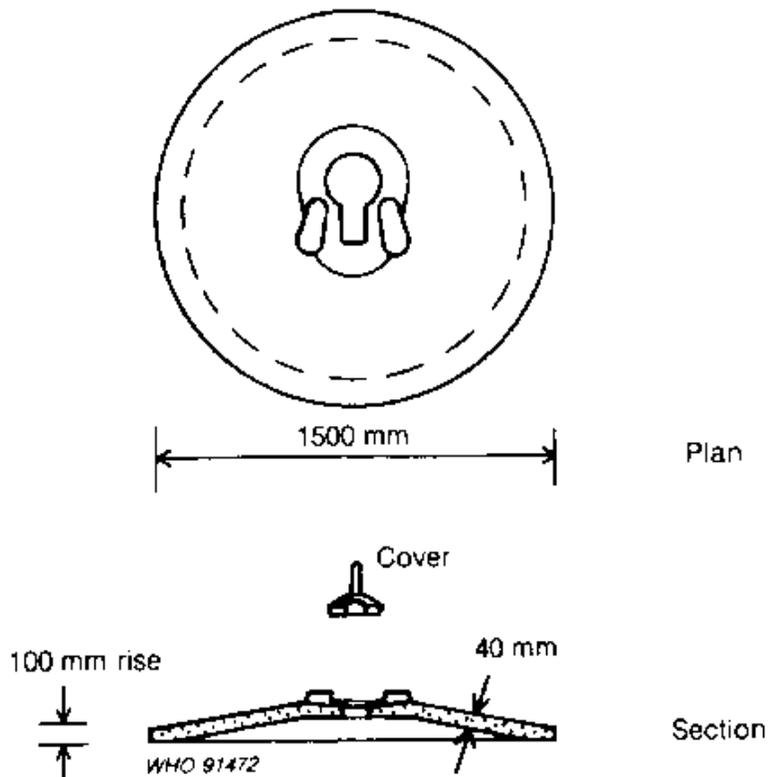
Although such domed slabs fall away from the centre, a small inward slope about 100 mm wide immediately around the squat hole is incorporated to direct any waste into the pit. These slabs have been used most effectively in areas with sandy soil which quickly absorbs any surplus wash water.
