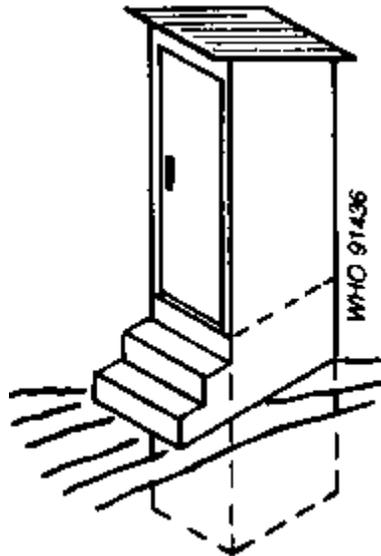
Raised pits can be used in combination with any other type of pit latrine (VIP, pour-flush, double-pit). A common application is where the groundwater level is close to the surface. A slight raising of the pit may prevent splashing of the user or blockage of the pit inlet pipe by floating scum.
