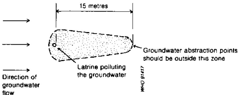
**Fig. 5.3. Protecting a hand pump from the pollution from a pit latrine**
