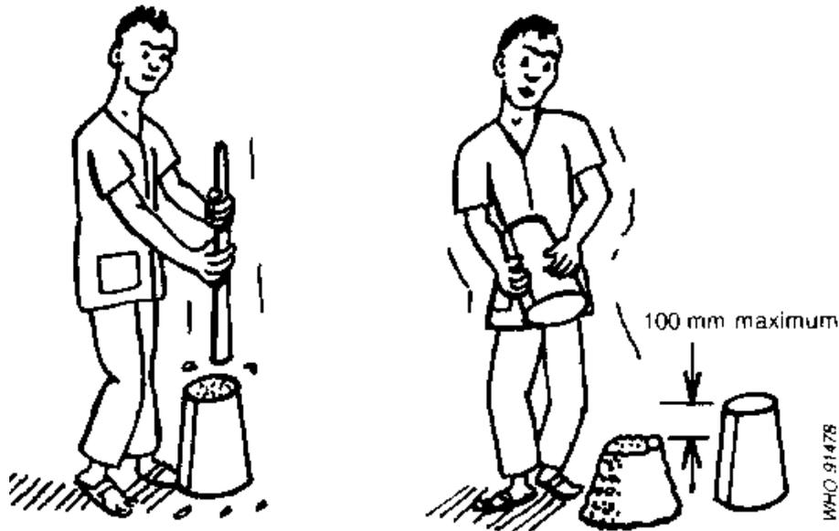
To check that the calculated amount of water is correct, a trial mix may be prepared and a slump test carried out. In this test, the concrete mix is compacted into a slump cone (Fig. 7.18), which is similar to an upturned bucket 300 mm high with the base removed. When the cone is removed, the concrete will slump, i.e., reduce in height; the maximum slump, for concrete that is to be reinforced, should be about 100 mm, and less for unreinforced concrete.
