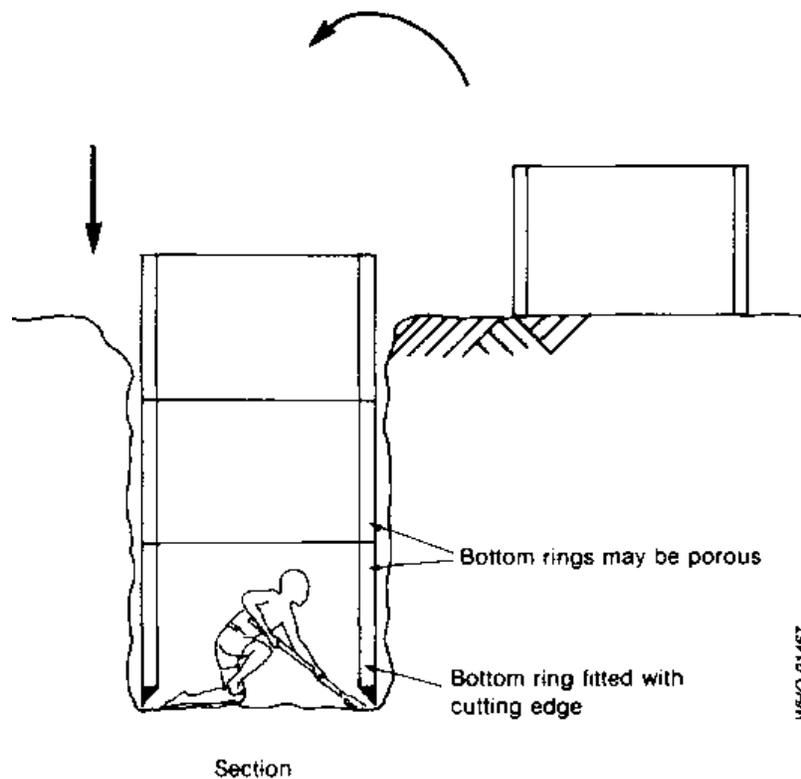
This method may also be used for linings of bricks or blocks. However, the lining must be constructed sufficiently far above the ground to ensure that the mortar has fully set before the lining enters the ground. The honeycomb method of construction cannot normally be expected to have sufficient strength to be sunk as a caisson.
