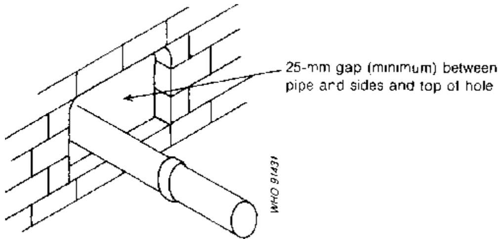
Fig. 6.13. Pipe fixed in place through a wall
