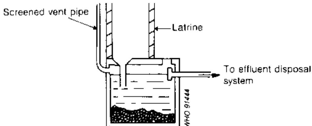
**Fig. 6.26. Aqua-privy with pan flushed by waste from a washing trough**
