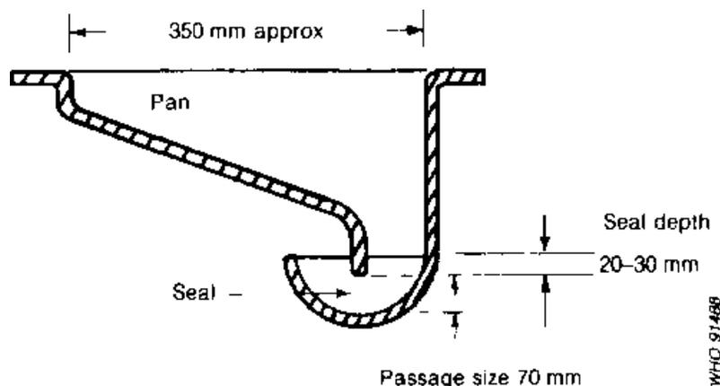
**Fig. 7.29. Pan and seal for offset pour-flush latrine**
