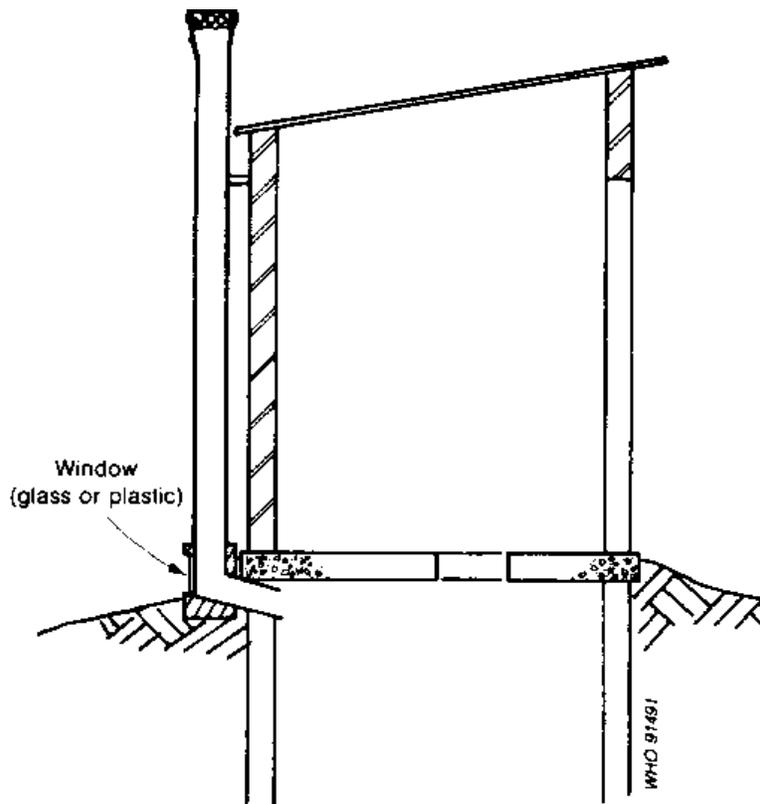
The draught through the vent is created primarily by the movement of wind across the top of the pipe. This air movement creates a suction effect, sucking air out of the pit and
