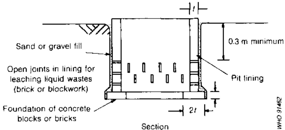
**Fig. 7.3. Lining for a shallow pit in soft ground**
