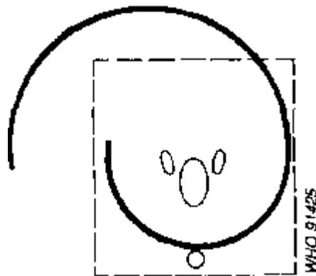
The superstructure can be constructed in the form of a spiral (Fig. 6.6). This excludes most of the light whether a door is fitted or not. The defecation hole must be left open to allow the free passage of air. The vent pipe should extend at least 50 cm above the latrine superstructure except where the latter has a conical roof, in which case the pipe should extend as high as the apex. Air turbulence caused by surrounding buildings or
