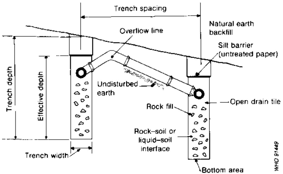
**Fig. 6.31. Drainage trenches laid in series in a drainage field. A-A indicates section shown in Fig. 6.30**
