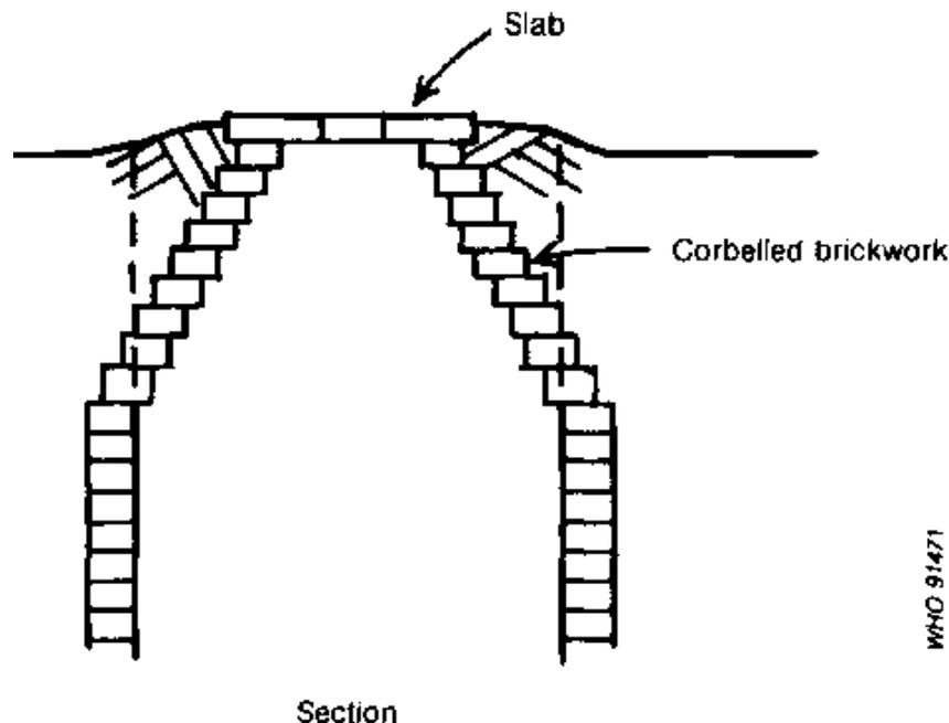
Slabs may be precast or constructed in situ, which means that the slabs are built over the pit, exactly where they are to be used. In a large agency-assisted programme, slabs are often manufactured at a convenient construction site away from the latrines and then brought to the site and laid across the pits. Where slabs are to be moved, weight and shape are both significant factors.
