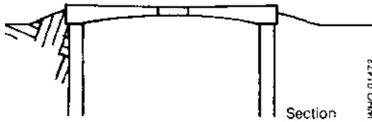
**Fig. 7.14. Arched brickwork lining and support**
