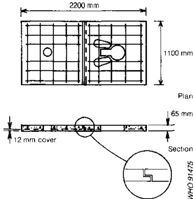
When individual bars are used, some may be omitted by mistake. One way of avoiding this is to use steel mesh, which consists of smaller diameter bars welded together. This can be cut to the required shape but there is likely to be wastage of the off-cuts that have to be discarded. A mesh with 7-mm bars at 200-mm centres, with a cross-sectional steel area of 193 mm<sup>2</sup>/m (yield stress 485 N/mm<sup>2</sup>) is normally sufficient.
