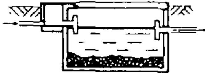
septic tank • Watertight chamber for the retention, partial treatment, and discharge for further treatment, of sewage
