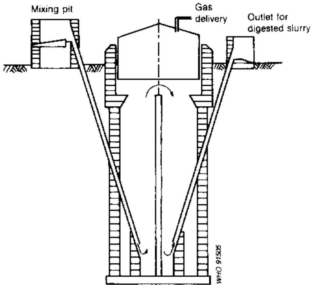
**Fig. A1.6. Biogas plant with fixed dome**
