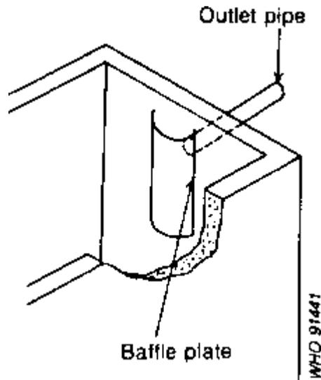
**Fig. 6.23. Septic tank outlet using full width weir**
