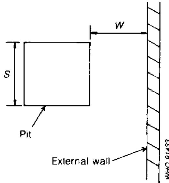
$W = \text{depth of pit or } 1.0 \text{ m provided } S \text{ is } 1.0 \text{ m or less}$
