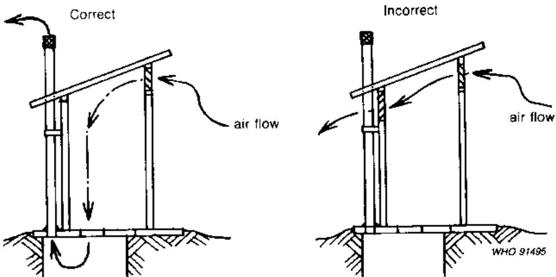
The superstructure must be strong enough to support a vent pipe extending 500 mm above the roof line. Alternatively it may be found that a block or brick vent adds rigidity to the superstructure.
