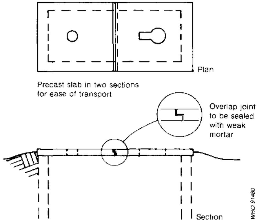
**Fig. 7.21. Circular slab for ease of transport**
