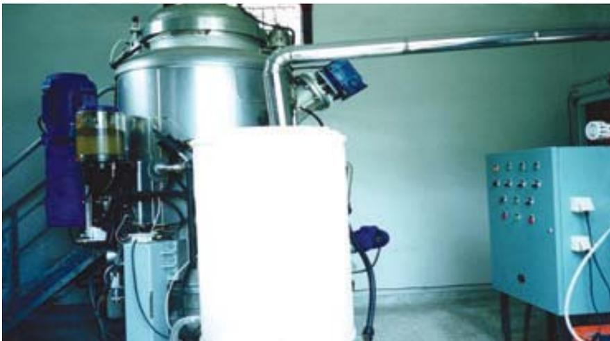
*Figure 8. Steam disinfection system with shredder*
