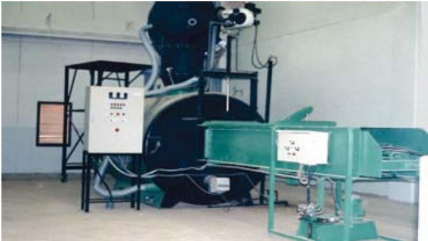
*Figure 7. High temperature double chamber pyrolytic incinerator*
