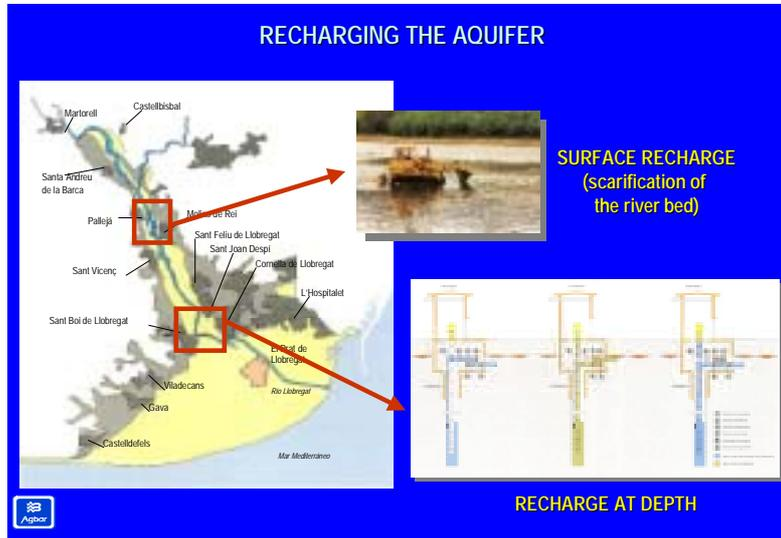
Recharge of the aquifer is undertaken through surface recharge, particularly where the aquifer is easily accessible through the riverbed. Besides the mechanical maintenance of the riverbed, the following issues are being considered: flow 10 – 35 m<sup>3</sup>/s,
