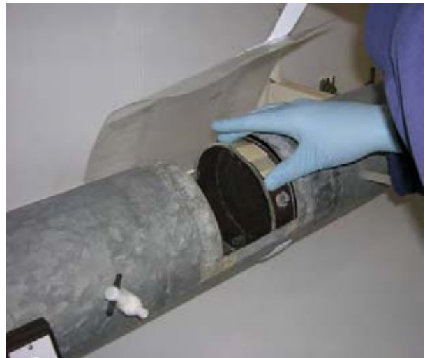
Figure A3.4. Sealed cage being positioned in wind tunnel (courtesy of Dr Jane Bonds, Florida A&M University, Panama City, Florida, USA)
